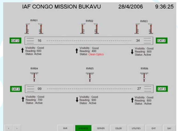
Runway Visual Range Display with support for two runways per module and up to eight individual sensor locations.
