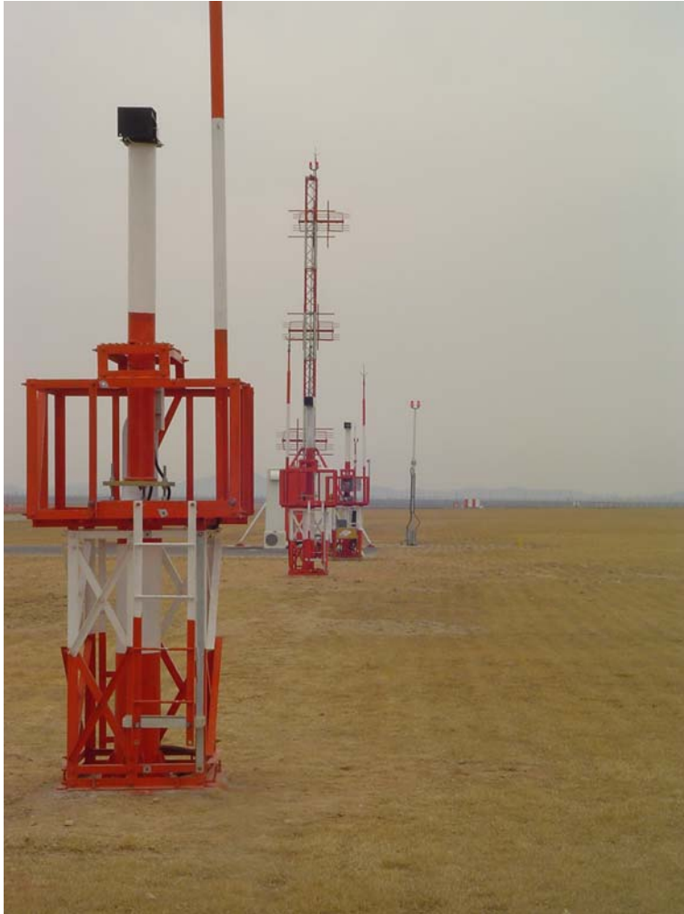
The MTECH 5000-200-D R5 Transmissometer Sensor in operation supplying CAT-3B operational data to on runway III at Incheon International.
