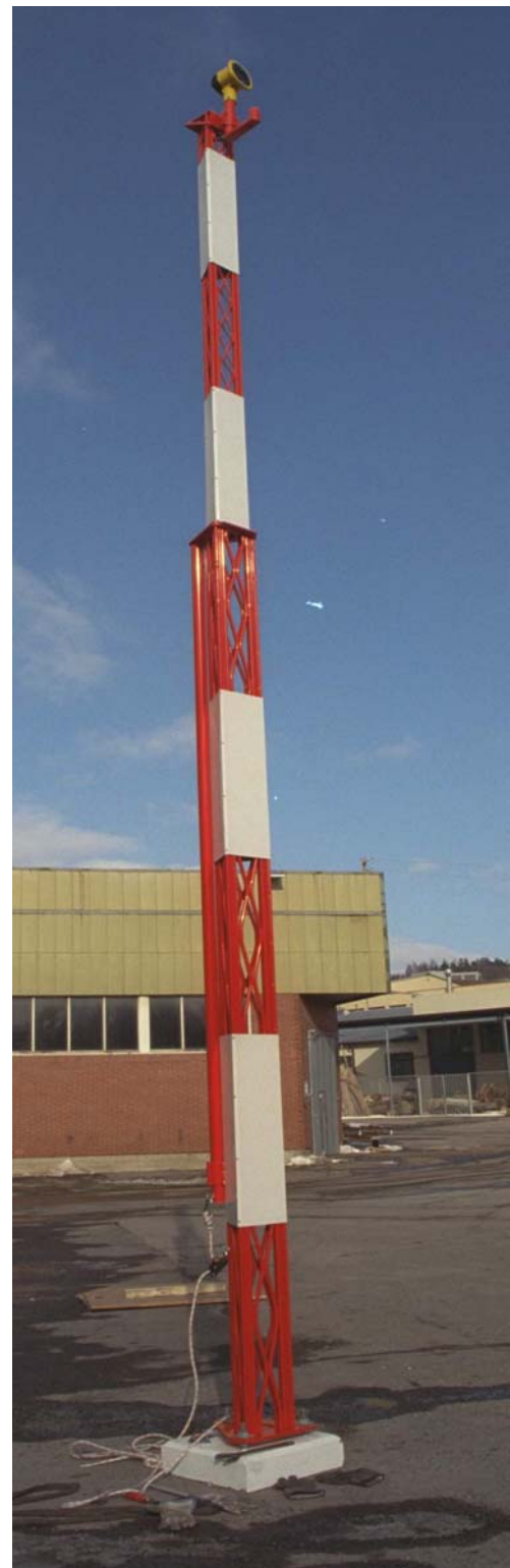
Frangible Mast undergoing factory pre-delivery test.
