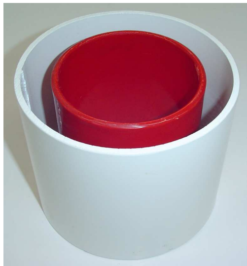
Example cross section showing dual frangible mast allowing for minimization of wind effects on central sensor shaft (shown in red).
