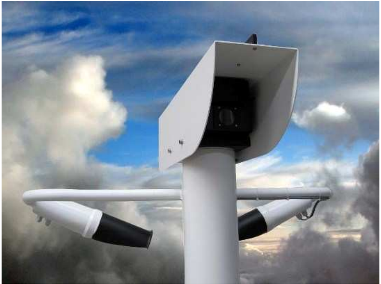
View of the 5000-200-EMOR Extended MOR Transmissometer with co-located 80km range forward scatter visibility sensor.
